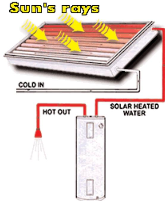
A solar water heater. Image, Sharpe Solar)
