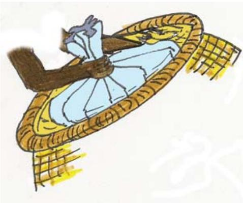
4. Open out the bag and tuck the edges of the cloth down between the insulating material and the inside of the basket. Stitch the cloth to the top rim of the basket.
