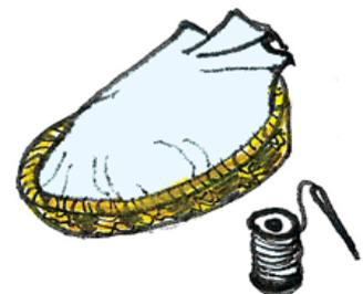
**Optional extra.** Add a shiny lining like aluminium foil or mylar to the pot's nest to reflect the radiant heat back into the pot. This works best when the pot fits snugly into the insulation with no air in between. This will also help keep the insulation dry, so that it does not need to be replaced as often.
