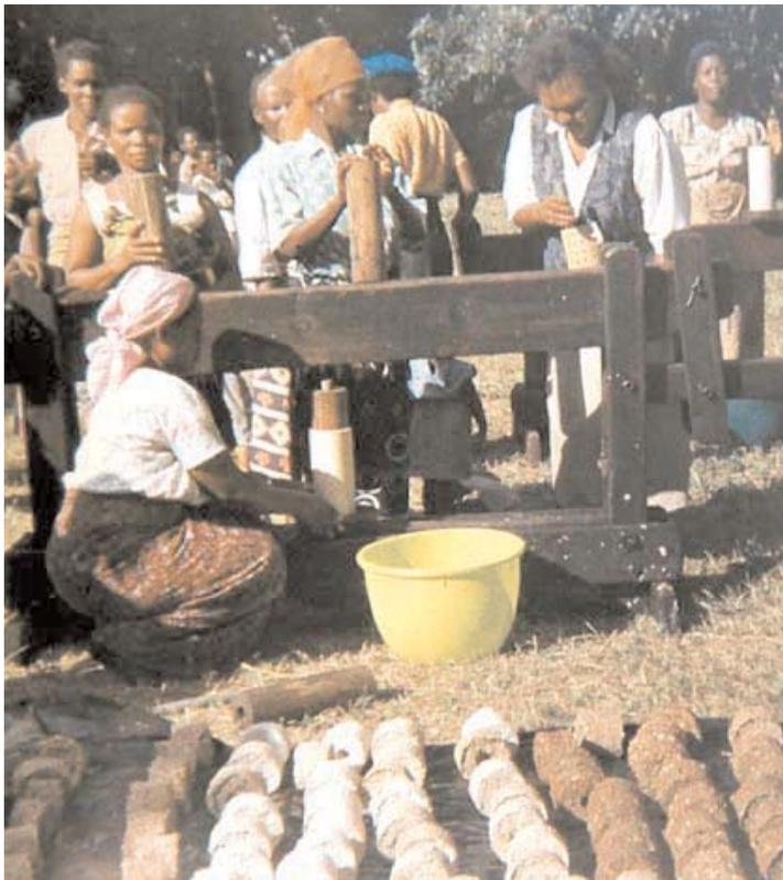
Hollow core briquette making process. Image, The Legacy Foundation.
